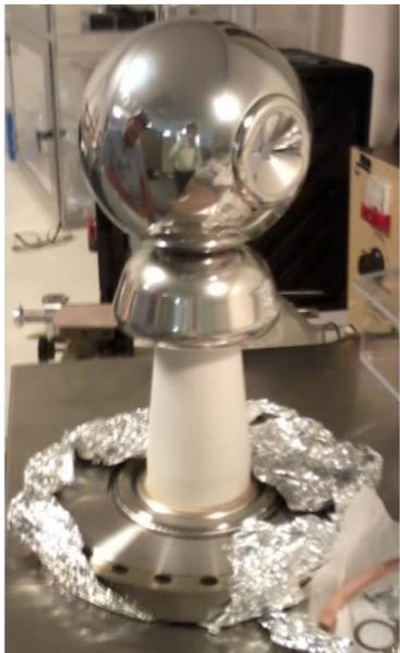
R30 with shielding electrode reached 375 kV
