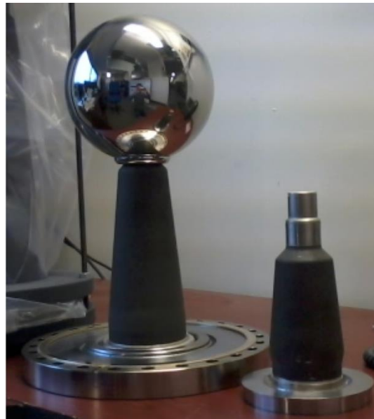
R30 with no shield arced at 325 kV
