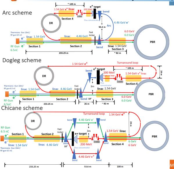
CDR: FCC-ee Injector complex is based on the SuperKEKB scheme with fixed target (has a hole for e- beam passage)
