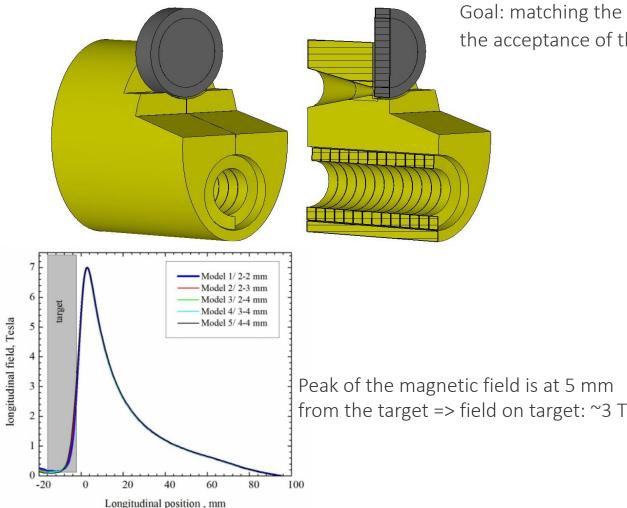
Goal: matching the e+ beam (with very large transverse divergence) to the acceptance of the capture linac.
