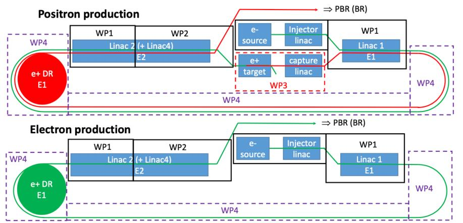
A full injector energy (6 or 20 GeV) can be used for the positron production
