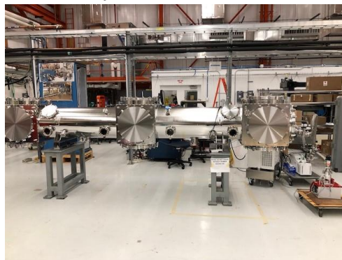
Cryostat vacuum vessel
