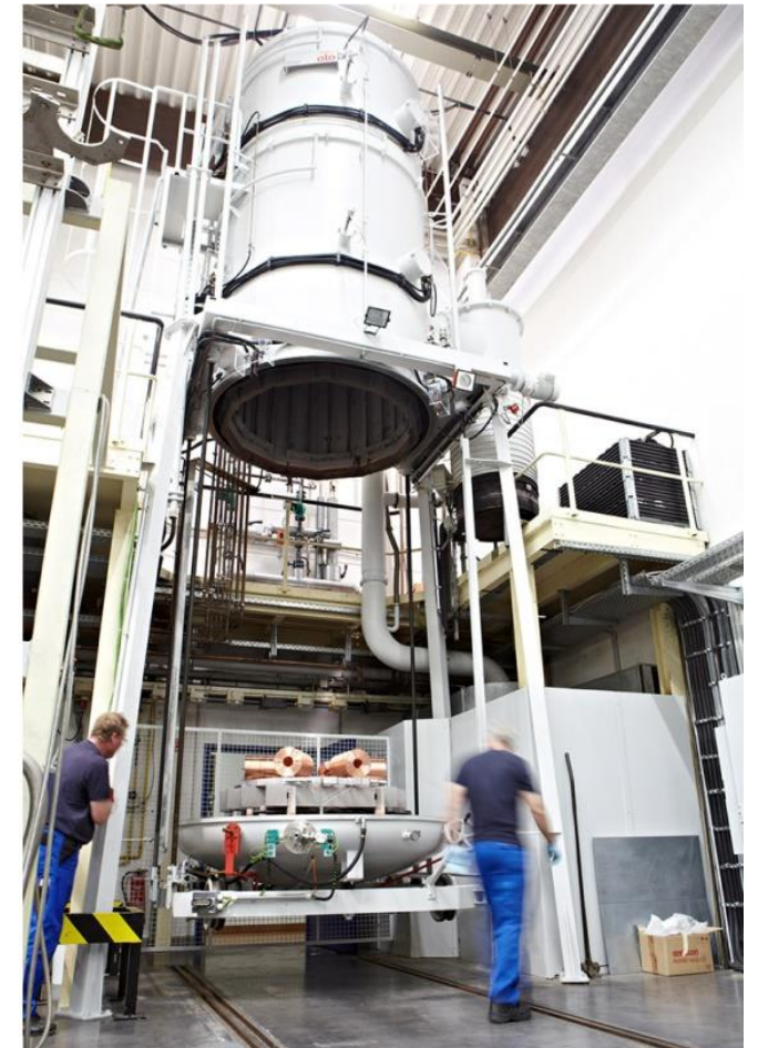
Heat treatment, vacuum brazing
