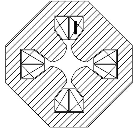
We remark that if  $l$  is the magnet length we are neglecting the losses in the coil ends: for a short magnet these can be as large (or even larger) than the losses of the “active field part”.
