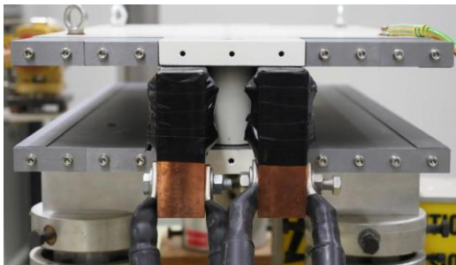
Prototype 1m-long, single busbar “coil”, measurements reported in [4]
