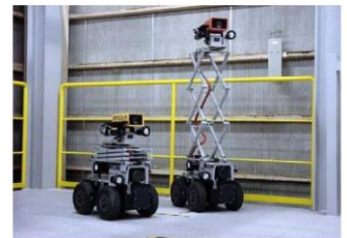
Figure 19 TALON equipped with rad-mapping system ©TEPCO
