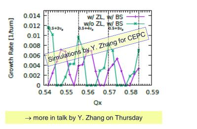
Longitudinal impedance leads to a spread of synchrotron tunes. As a result, the good regions for  $Q_{\rm x}$  shrink.
