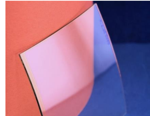
Curved ITO coating on glass following a tempering and bending process at 650 °C (Fraunhofer IST)
