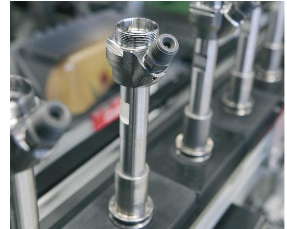
With HiPIMS, Bosch achieves higher component quality with increased process reliability in the production of common rail injectors
