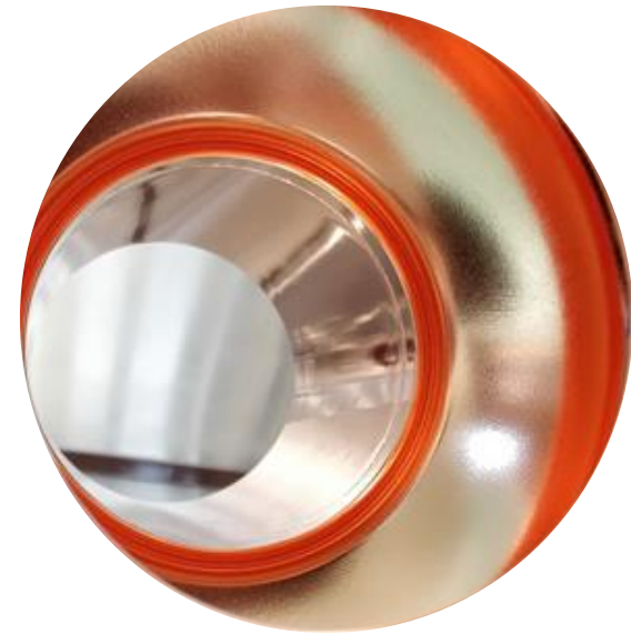
Surface state of an electropolished 1.3GHz cavity
