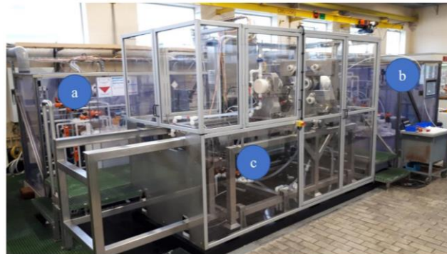
a) Copper chemical plant; b) niobium chemical plant; c) cavity handling device
