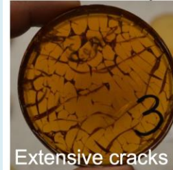
CTD-101 k, used by US LARP, after one thermal cycle to 77 K
