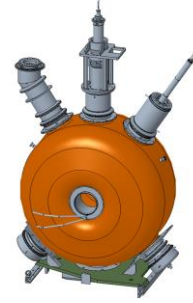
Hadron - 197 MHz bunch compression cavity
