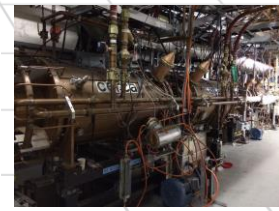
Hadron - 24.5 MHz acceleration cavity
