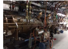
Hadron - 24.5 MHz acceleration cavity
