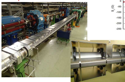
Permanent magnets for beam pipes at drift spaces
