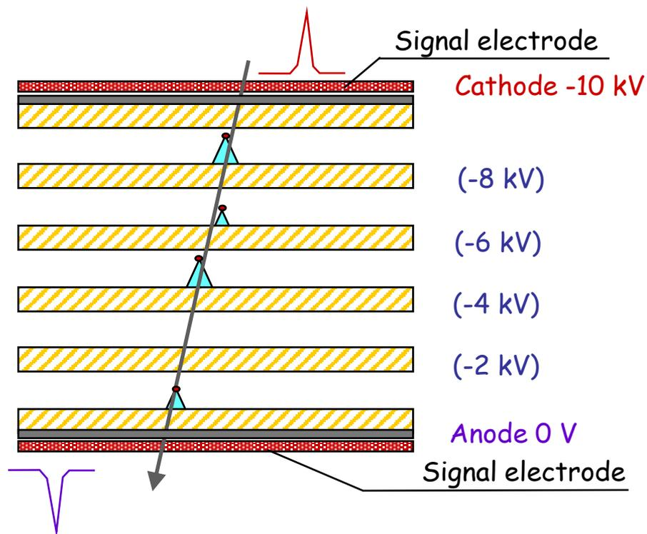
Stack of equally-spaced resistive plates with voltage applied to external surfaces (all internal plates electrically floating)
