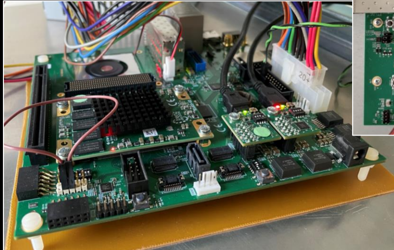
Trenz mezzanine + carrier board (TE0803 + TEBF0808)
