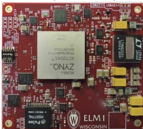
Embedded Linux Mezzanine (ELM) ELM1 (XC7Z045-based)
