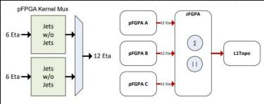
pFPGA ⇄ zFPGA connection is GTH/GTY UltraScale+ GTH (16.3Gb/s) UltraScale+ GTY (32.75Gb/s)
