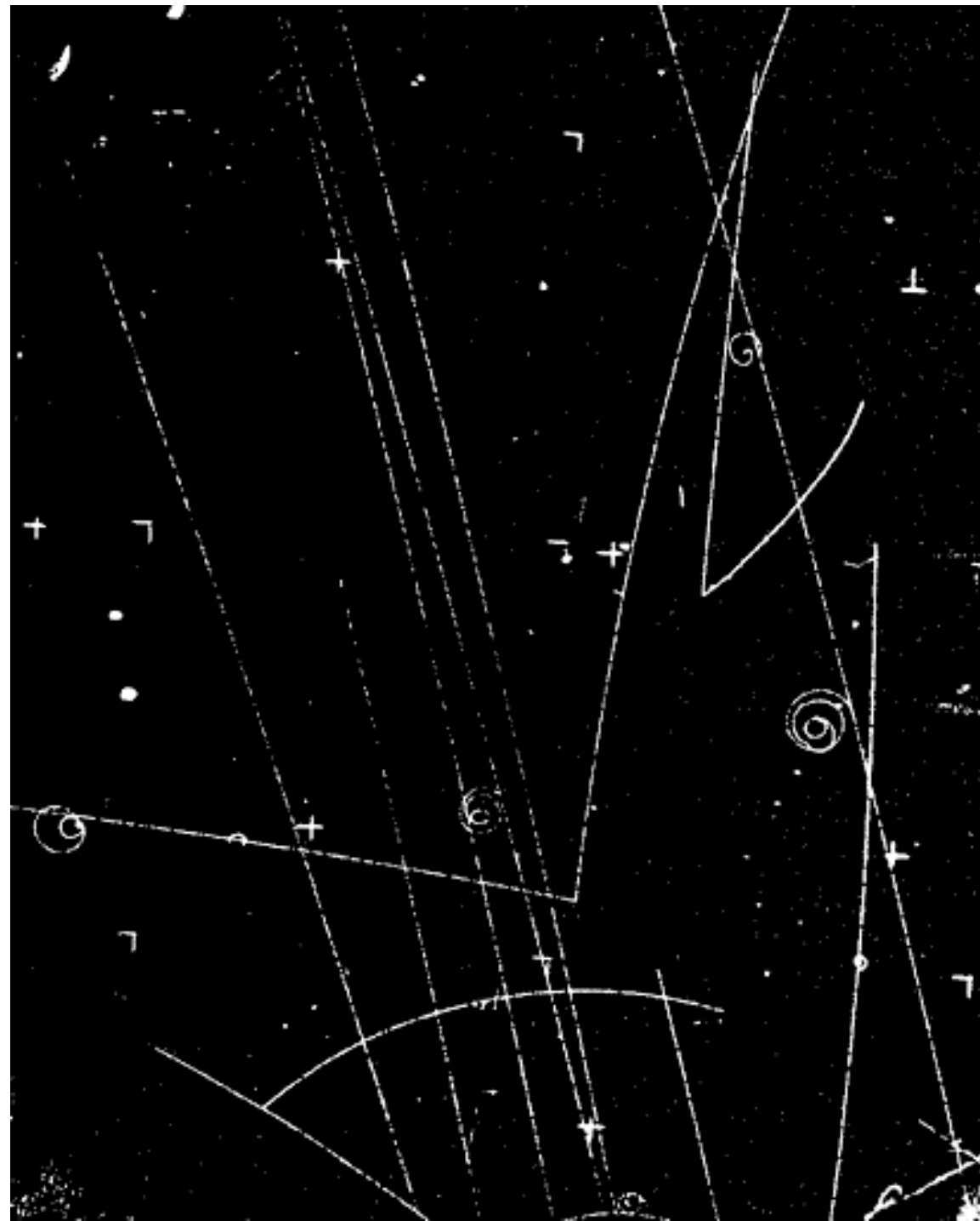
Interaction in a liquid hydrogen bubble chamber at the Berkeley Bevatron accelerator. http://www.hep.fsu.edu/~wahl/phy4822/expinfo/BC/bubchamber.html
