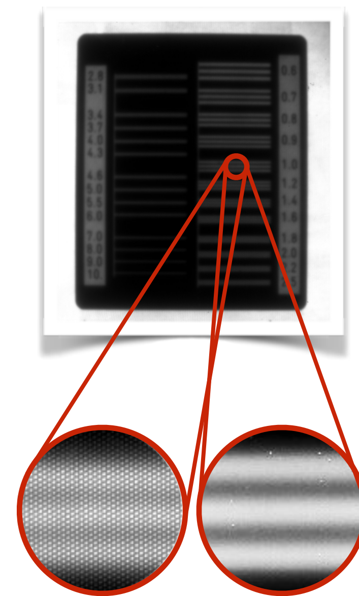
Triple-GEM Hole structure
