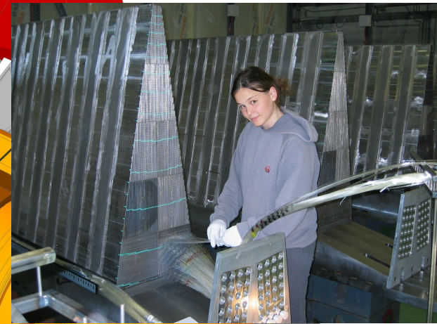
FORWARD CALORIMETER Steel + Quartz fibres ~2,000 Channels
