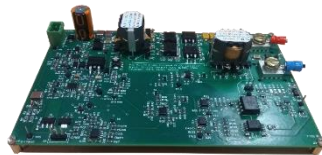
12V DC/DC demo board
