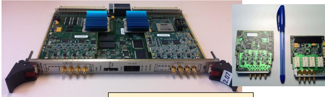
PSB LLRF electronics (RF and FPGA)
