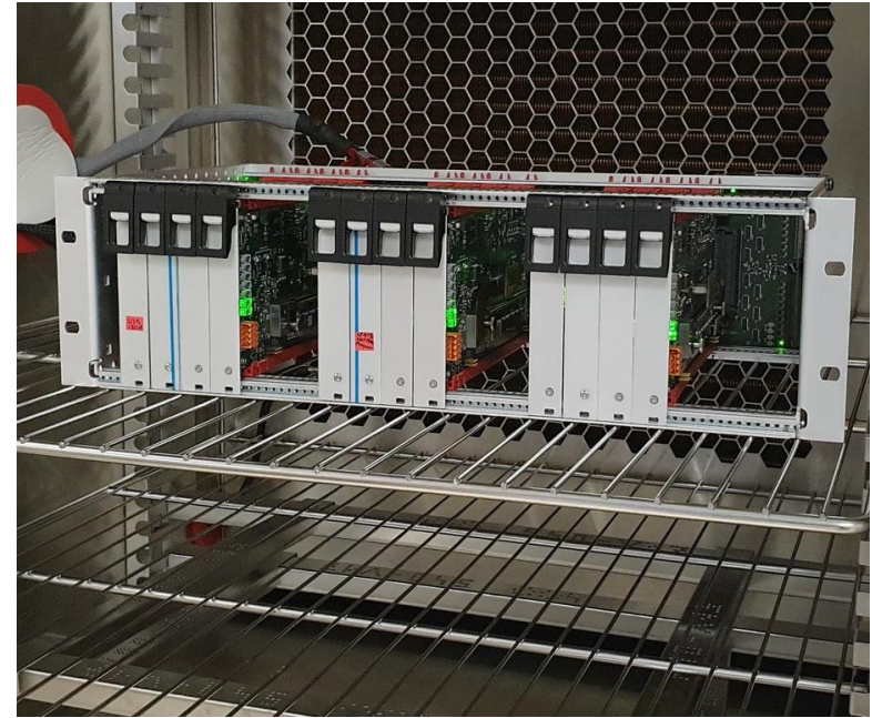
Test crate in the climatic chamber during the cold testing
