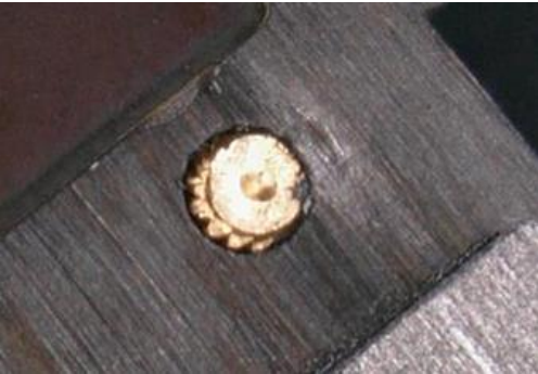
Solution: gold plated aluminium inserts are press fitted into the CF stiffeners and connects them to the hybrid's GND
