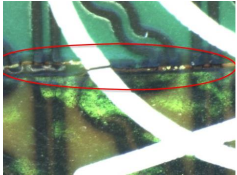
Crack in the soldermask in the transition zone between soldermask and coverlay
