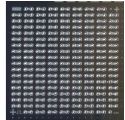
Daisy-chain test flip-chip with 254 \mu m pitch.
