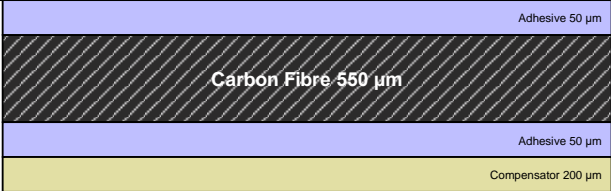
Build-up specification of the 2S-SEH
