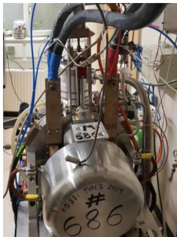
Carburization pumpstand w. new control software
