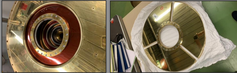
REX Linac 9Gap anodic capacitor repair (courtesy C. Gagliardi)
