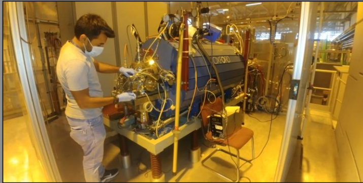
Installation new E-gun at REX EBIS (courtesy G. Kathri, F. Wenander, S. Mataguez)
