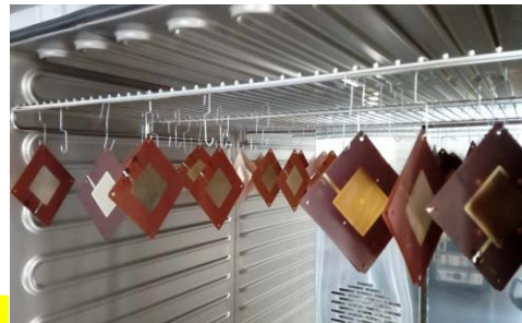
A SET OF SMALL THGEMS PREPARED AND CHARACTERIZED FOR SYSTEMATIC H-ND STUDIES
