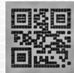
Micro QRcode ( 750 \mu\text{m} \times 750 \mu\text{m} )
