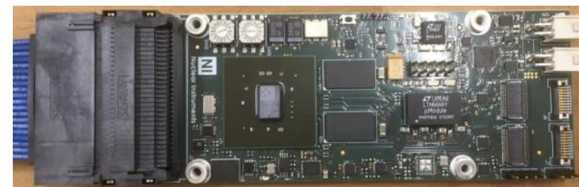
Readout electronics developed by Nuclear Instruments
