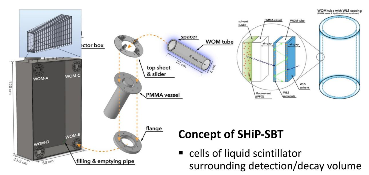
light readout via Wavelength-shifting Optical Modules (WOMs) and SiPMs
