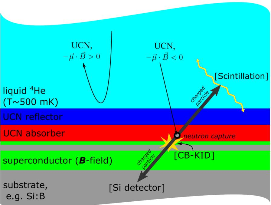
Ultracold neutron (UCN) detection with polarization-sensitivity, via applied magnetic fields partially cancelling the neutron-optical potential for one spin state. Various readout mechanisms to be explored.
