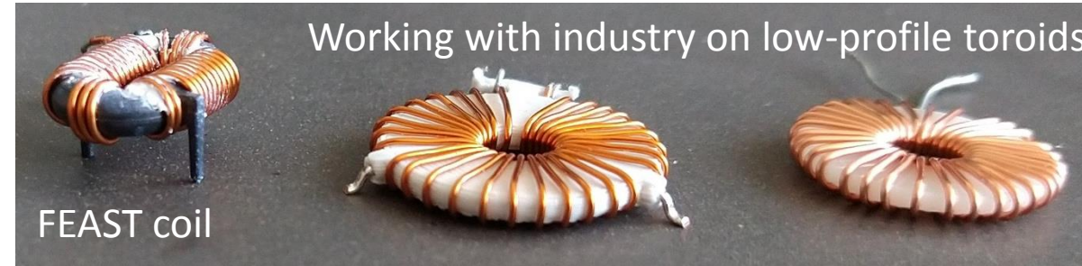
Prototype in-PCB inductors
