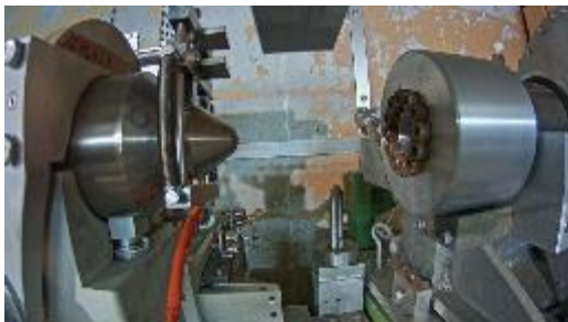
Temperature sensor installation on AD target
