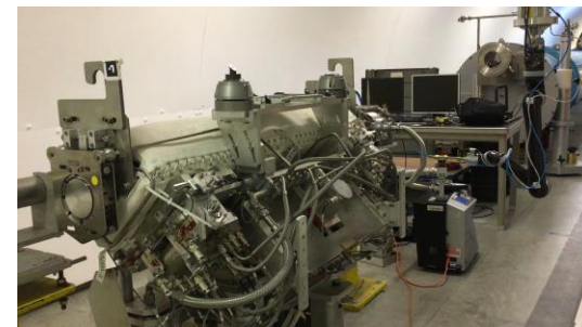
Remote Vacuum Leak detection
