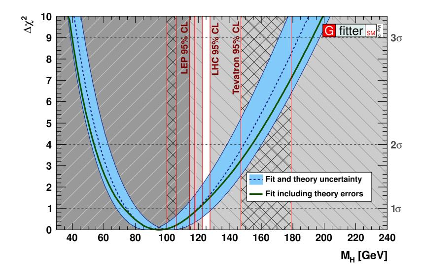
The blue band, which does not employ the direct Higgs search limits, corresponds to a upper bound of  $m_h < 153$  GeV at 95% CL. A similar result of the LEP Electroweak Working group quotes  $m_h < 152$  GeV at 95% CL.
