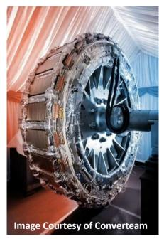
AMSC 36.5 MVA, 6 kV 120 rpm 8 poles, 75 tons Efficiency > 97 % Dimensions: 3,4 m x 4,6 m x 4,1 m
