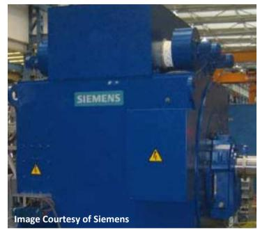
Siemens 4 MW, 3.1 kV 120 rpm, 320 kNm 37 tons 50 km HTS Test in 2010
