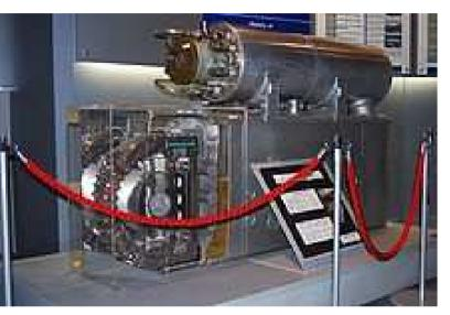
Superconducting magnet and a liquid helium tank on top of it
