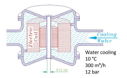
Power Supply 6 MW (20 kA, 300 V) 20 T NTSL-Magnet (KIT)
