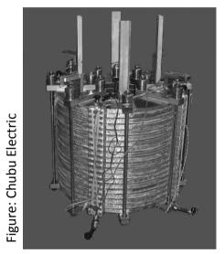
1 MJ , 1 MW Bi 2212 tape 500 A, 5 K conduction cooled Voltage: 2.5 kV KERI, Korea Power quality
