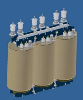
1 MVA Demonstrator 11 kV/415 V Primary YBCO Secondary YBCO Roebel cond. Test in 2013 2 MVA Demonstrator 22kV/6.6 kV Primary Bi 2223 tapes Secondary YBCO tapes Successful test in 2009 28 MVA Prototype 69 kV Primary and secondary with YBCO tapes Test planned in 2013
