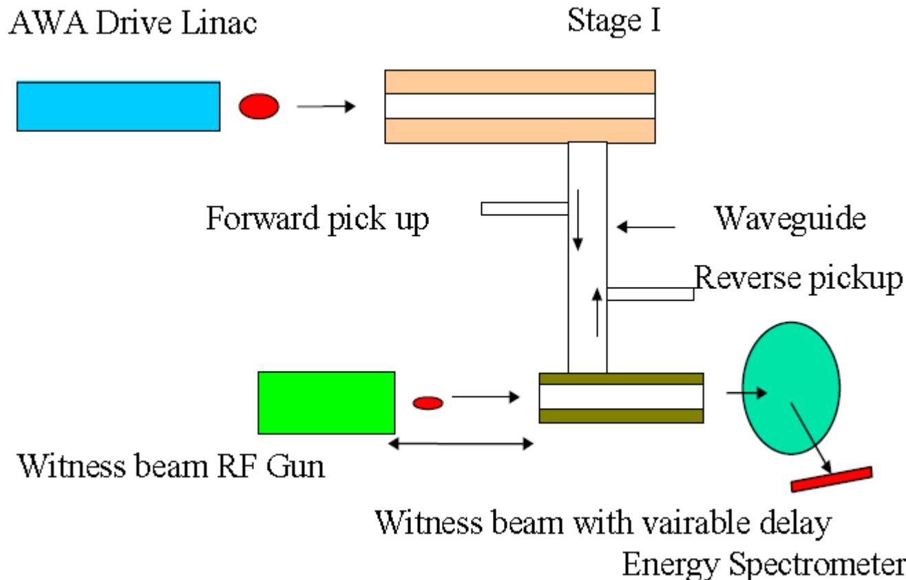
Witness and drive bunches are moving along the different structures
