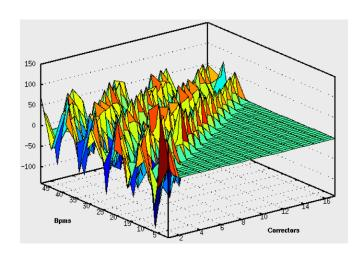
(Above) Measured Rx response matrix for the test-section of the linac (17 correctors, 48 BPMs)
