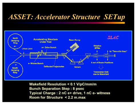
$ightharpoonup W_{\perp}$  is the transverse wake function at time t behind the drive bunch,  $E_{w}$  (~1.2 GeV) is the witness bunch energy and  $\Delta y_{d}$  is the offset in the drive bunch from the electrical centre of the accelerating structure.
