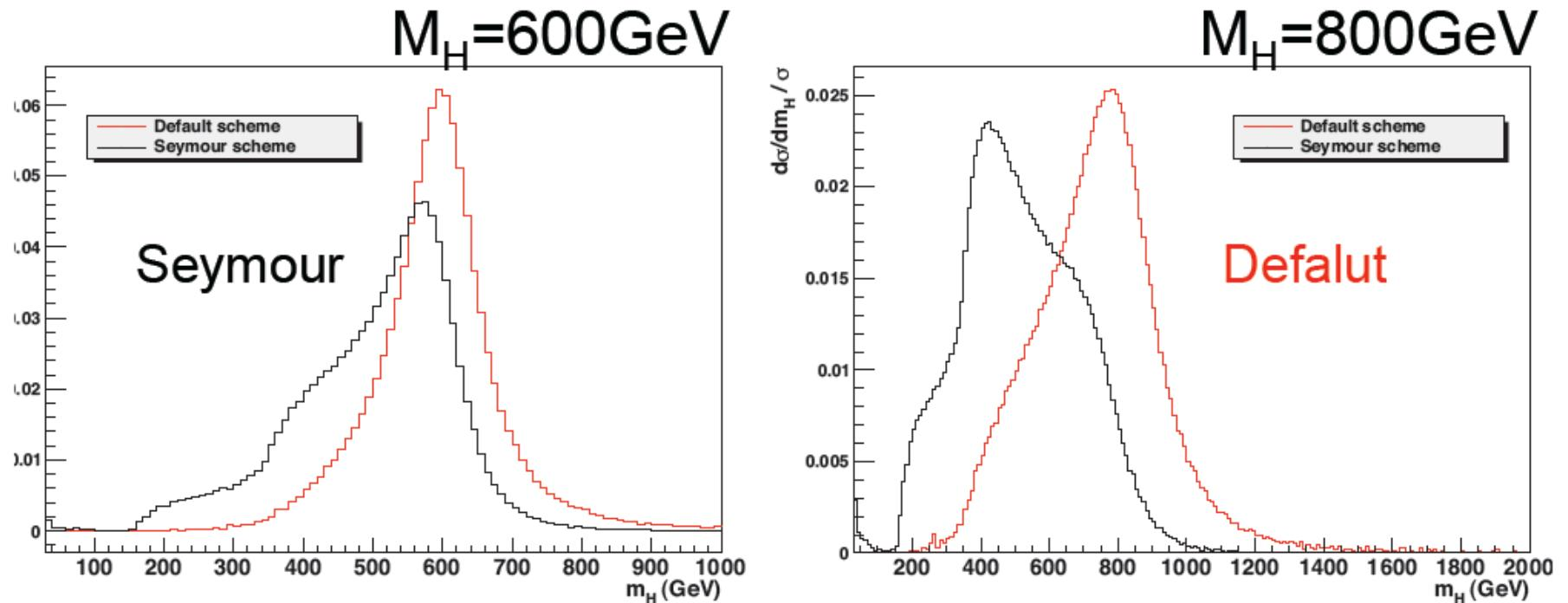
ISA includes non-resonant contributions, which “default” does not. Meaningless to compare shapes, but absolute  $\sigma$ s should agree near resonance
