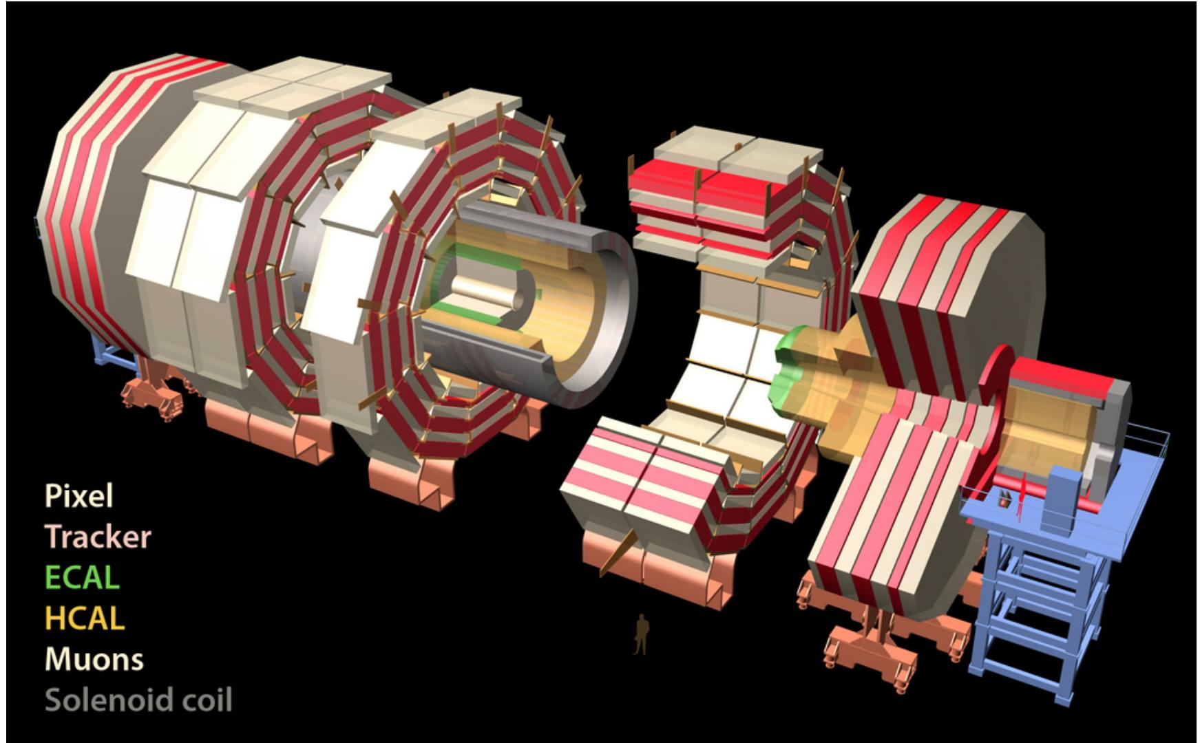
Silicon tracker (pixels+strips)      Lead tungstate crystal ECAL
