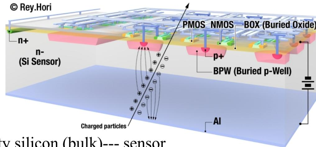
High resistivity silicon (bulk) --- sensor
