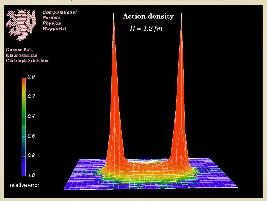
chromoelectric flux tube formation between the static quark-antiquark pair-> dual Meissner effect
