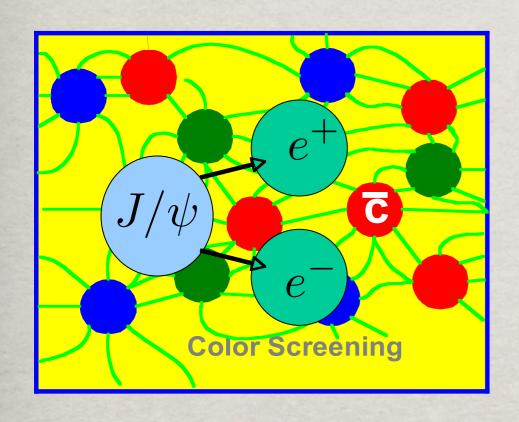
Debye charge screening  $m_D \sim gT$   $V(r) \sim -\alpha_s \frac{e^{-m_D r}}{r}$
