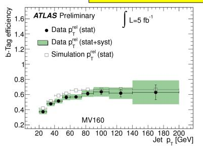
*b*-tagging efficiency of MV1 as a function of jet  $p_T$  at ~60% operation point.
