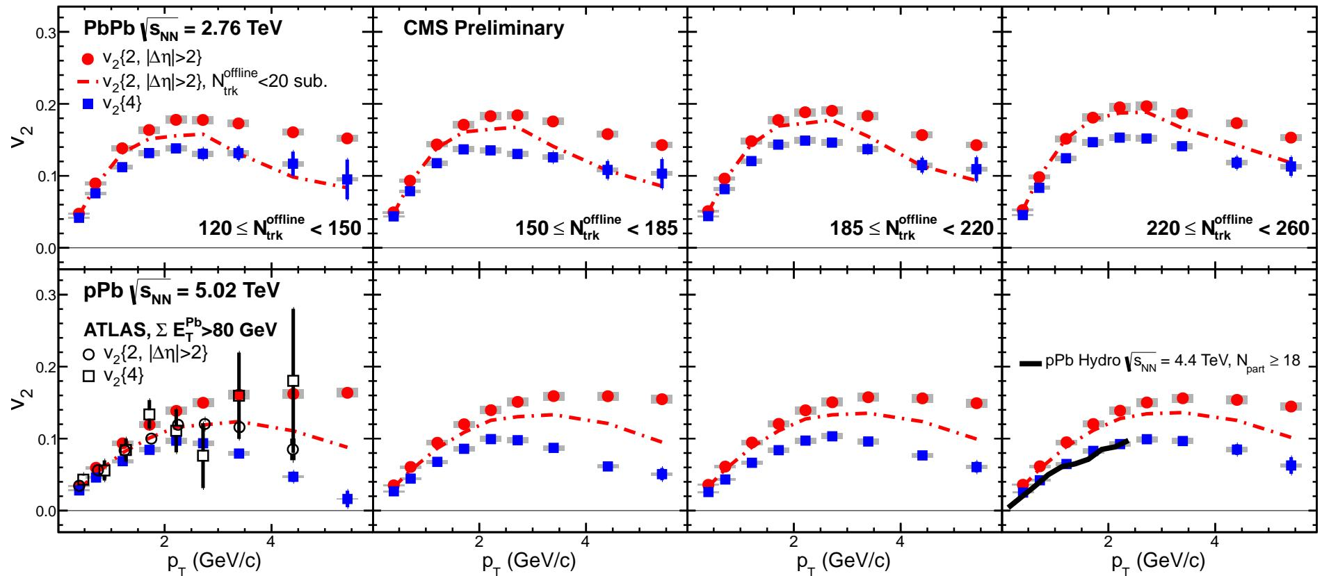
Fourier  $v_2$  from two- and four-particle analysis for the  $p_T$  range of 0.3-3 GeV/c
