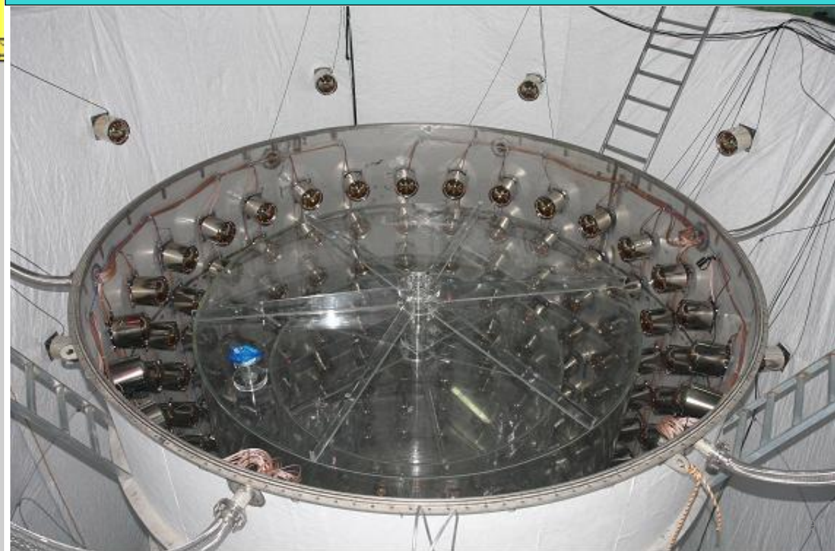
Finishing PMT installation (2011. 1)
