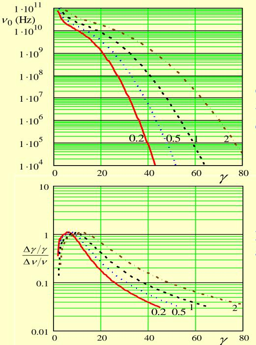
The mode frequency (top) and the relative accuracy of determination of  $\gamma$  (bottom). a = 3 cm, $\gamma = 0.5 \text{ mm},$  $r_0 = 0.5 \text{ mm}.$
