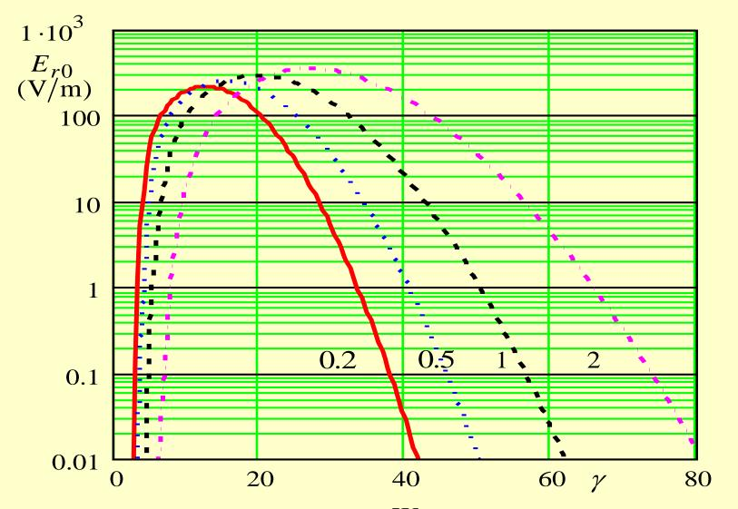
Amplitude of the component  $E_r^W$  on the outward surface of waveguide depending on  $\gamma$ ; magnitudes of  $d_{\phi}$  (cm) are indicated near the curves.
