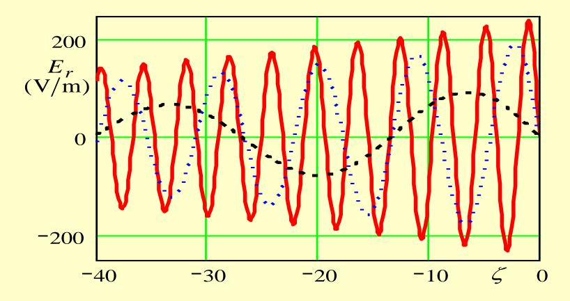
Typical wakefield. Component  $E_r^W$  on the outward surface of waveguide depending on the distance  $\zeta = z - Vt$  for  $\gamma = 15$  (solid red),  $\gamma = 20$ (dotted blue),  $\gamma = 25$  (dashed black). Conductivity of wires is  $5 \cdot 10^7$  (Om m)<sup>-1</sup> Other parameters are the same as early. 18
