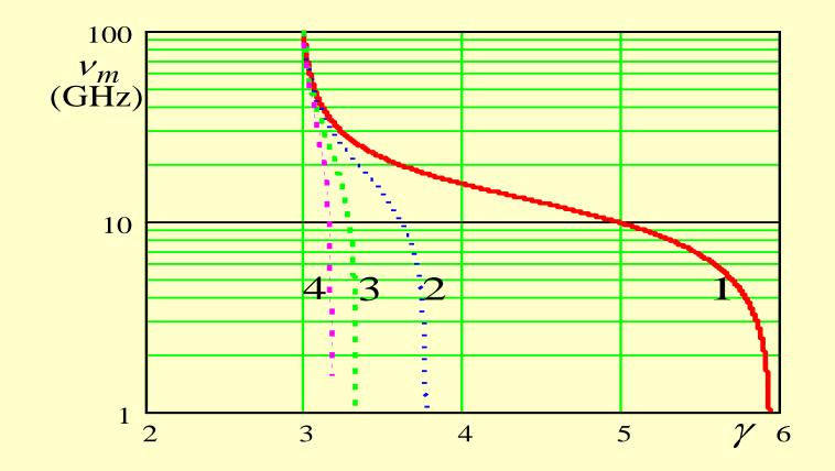
The mode frequencies depending on Lorentz factor; waveguide radius is 5 cm, coating permittivity = 5;  $r_0 = 0.2 \text{ mm}, \quad r_d = 0.3 \text{ mm}, \quad d = 10 \text{ mm},$ mode numbers are indicated near the curves. The 1<sup>st</sup> mode frequency depending on Lorentz factor; waveguide radius is 5 cm, coating permittivity = 5;  $r_0 = 0.2 \text{ mm}, d = 10 \text{ mm},$
