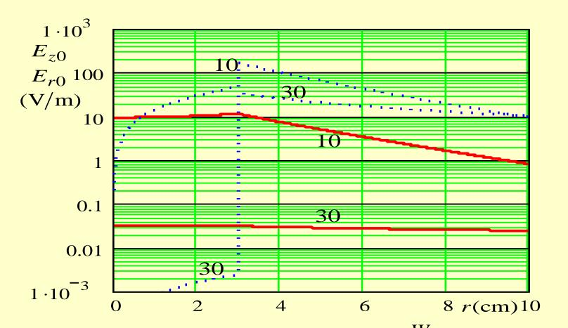
Dependency of amplitude of component  $E_z^W$  (solid red) and  $E_r^W$  (dotted blue) on distance from waveguide axis;
